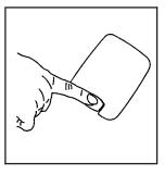
Press the area at the front of the handle located on the cover so that the back edge raises.
